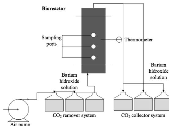
Fig. 1. Schematics of a bioreactor unit.
