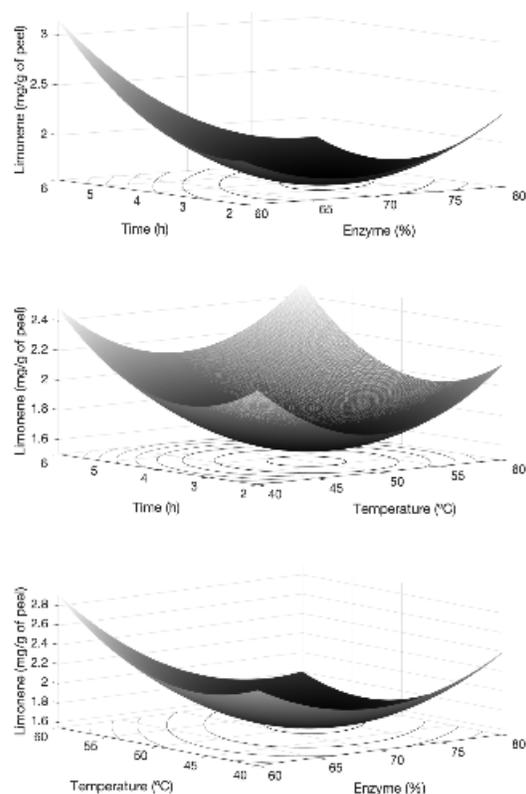
Fig. 2. Surface-response for extraction of limonene from limes peels.
