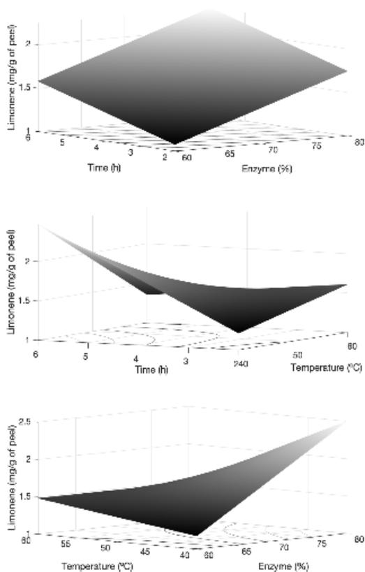
Fig. 1. Surface-response for extraction of limonene from orange peels.
