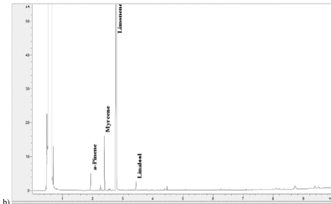
Fig. 3. Compound profile from orange peels obtained with: a) Commercial enzymes, b) blank.
