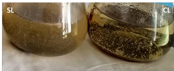
Figure 9. *Rhodococcus sp.* strain growing in suspended form in treatment without biosurfactant (SL) and stuck to oil in treatment with biosurfactant (CL).
