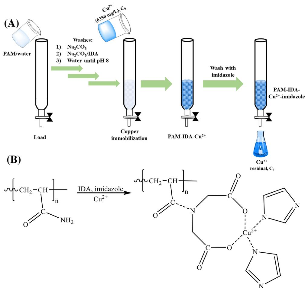
Fig. 2. Column preparation process (A) and mechanism of copper immobilization (B).
