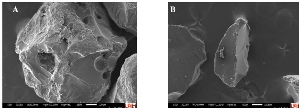
Fig. 3. SEM micrographs of polyacrylamide matrices: 6%T (A) and 10%T (B) at 100x magnifications.
