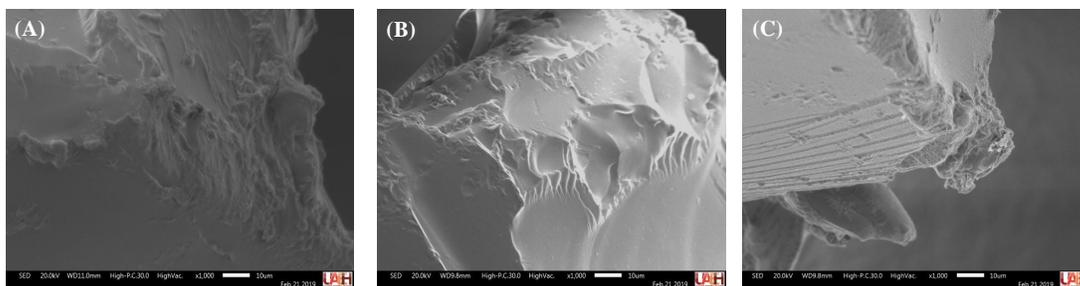
Fig. 4. SEM micrographs of PAM at 1000X magnifications of: (A) PAM at 10%T, (B) PAM-IDA-Cu<sup>2+</sup>, and (C) PAM-IDA-Cu<sup>2+</sup>-imidazole.
