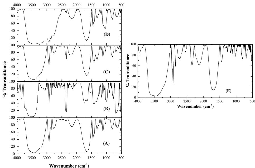
Fig. 5. FT-IR spectra of PAM 10 %T (A), PAM-IDA (B), PAM-IDA-Cu<sup>2+</sup> (C), PAM-IDA-Cu<sup>2+</sup>-imidazole (D) and PAM-IDA-Cu<sup>2+</sup>-imidazole after proteins desorption (E).
