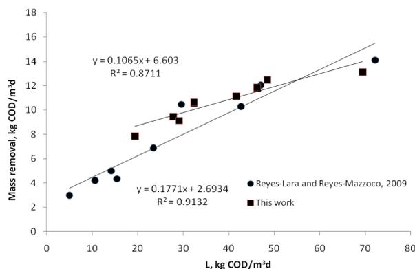
Fig. 3. Effect of organic load in the mass removal efficiency of organic matter, from the results of organic matter removal (Table 2).
