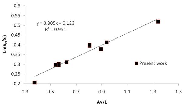
Fig. 2. Evaluation of the kinetic constant with the Eckenfelder model, Eq. 1, from the results of organic matter removal obtained at 55 and 79-cm packing depth (Table 2).
