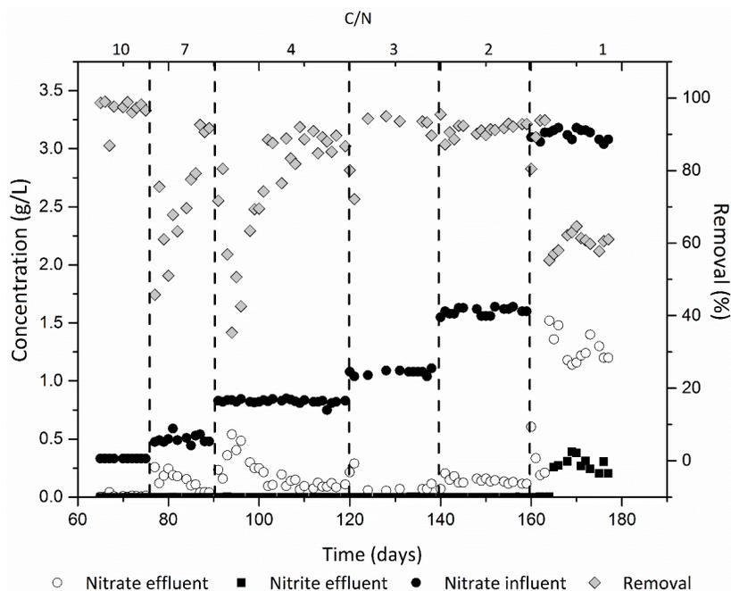
Fig. 3. Nitrogen removal in the reactor at different C/N ratios during the experiment.
