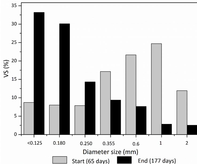
Fig. 6. Granulometry made at the beginning and end of simultaneous denitrification and methanogenesis process.
