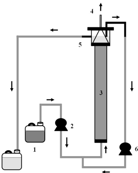
Fig. 1. Experimental set-up of the anaerobic expanded bed reactor. (1) Feed tank, (2) feed pump, (3) reactor, (4) biogas outlet, (5) effluent outlet, and (6) effluent recycling pump.
