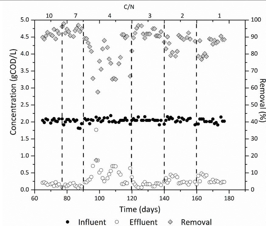
Fig. 2. Organic matter removal in the simultaneous denitrification and methanogenesis process.
